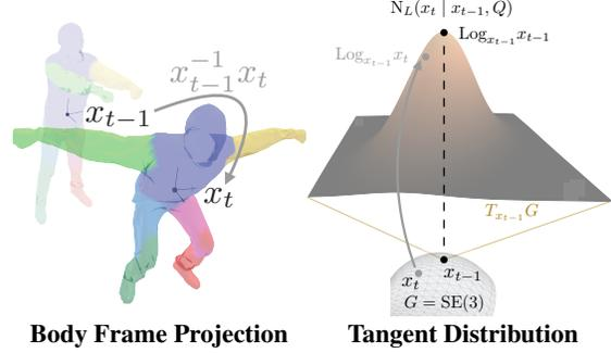
Figure 5. *Left:* Object dynamics of body frame at time  $t$  are projected into coordinates at time  $t - 1$  by the Lie group operation  $x_{t-1}^{-1} x_t$ . *Right:* The projection is in  $SE(3)$  with Gaussian statistics in the tangent plane of  $x_{t-1}$ . The figure notionally depicts two degrees of freedom, whereas  $SE(3)$  would have 6 degrees.
